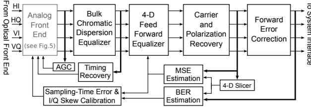
Fig. 4. Digital signal processor architecture for a DP-QPSK coherent receiver.
