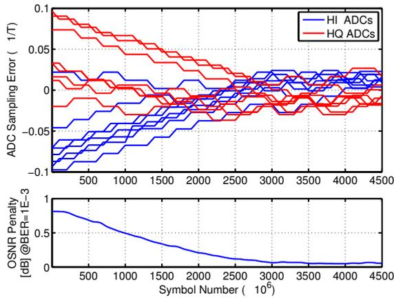
Fig. 6. Calibration convergence from an initial random set of sampling-time error and I/Q TS. M-MSE calibration with  $OSNR = 13dB$ . Top: ADC phase errors for polarization H. Bottom: OSNR penalty at  $BER = 10^{-3}$
