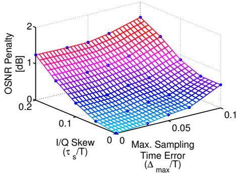
Fig. 3. OSNR penalization at  $BER = 10^{-3}$  as a function of the maximum sampling-time error ( $\Delta_{max}$ ) and the I/Q timing-skew.
