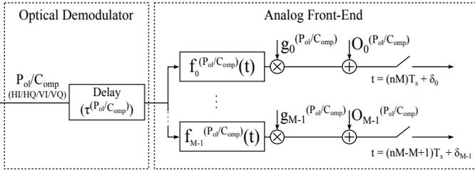
Fig. 2. Channel model of one of the four channels (HI, HQ, VI, VQ).
