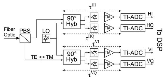
Fig. 1. Optical/analog front-end for a coherent optical receiver.
