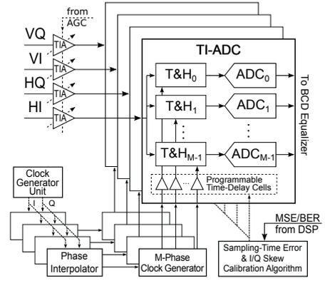
Fig. 5. Detailed block diagram of proposed Analog Front-End based in four TI-ADC with mixed signal calibration.
