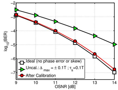
Fig. 7. Performance comparison of pre and post calibration with M-MSE.
